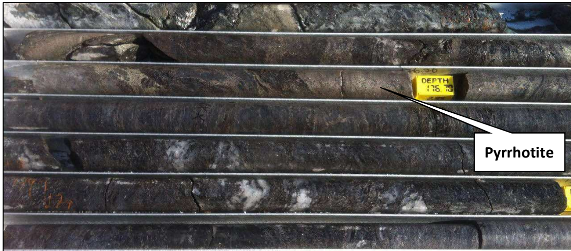
Figure 5: Section of core from the upper sulphide zone from 175m in KNDD001. Note the zones of semi-massive pyrrhotite associated with ultramafic rock types. This style of sulphide mineralisation is visually similar to the host sulphides of Ni+Cu+Co+PGEs at the Maibele North Resource some 23km to the southwest.
