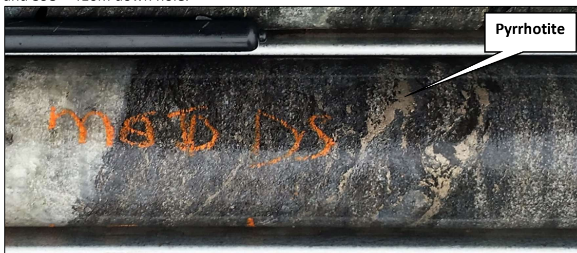
Figure 3: Examples of the disseminated and stringer pyrrhotite mineralisation (bronze coloured mineral) in core from around 365m down hole in MTDD003.
