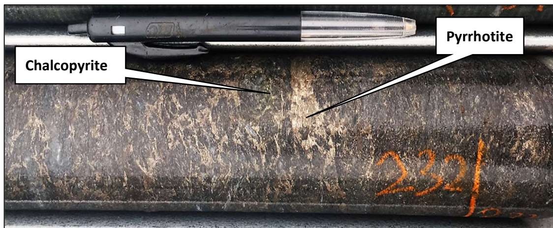
Figure 4: Examples of the 40cm zone of heavily disseminated pyrrhotite + chalcopyrite mineralisation in core from around 232m down hole in MKDD001. This style of sulphide mineralisation is visually similar to the host sulphides of Ni+Cu+Co+PGEs at the Maibele North Resource some 21km to the southwest.
