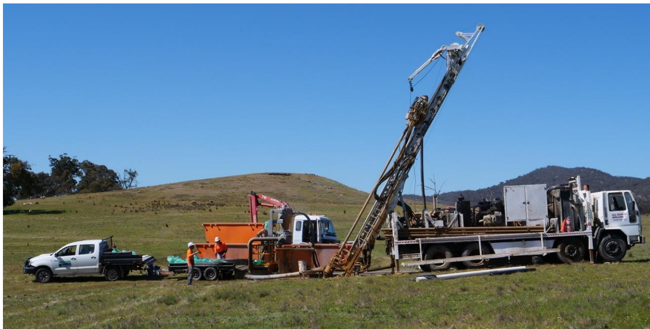
Figure 2: Reverse Circulation drilling underway at the Adventure Lode, at the Irvine Gold Project, October 2018.
