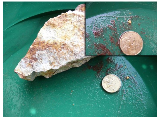
Photograph 1. Coarse gold from crushed sample.
