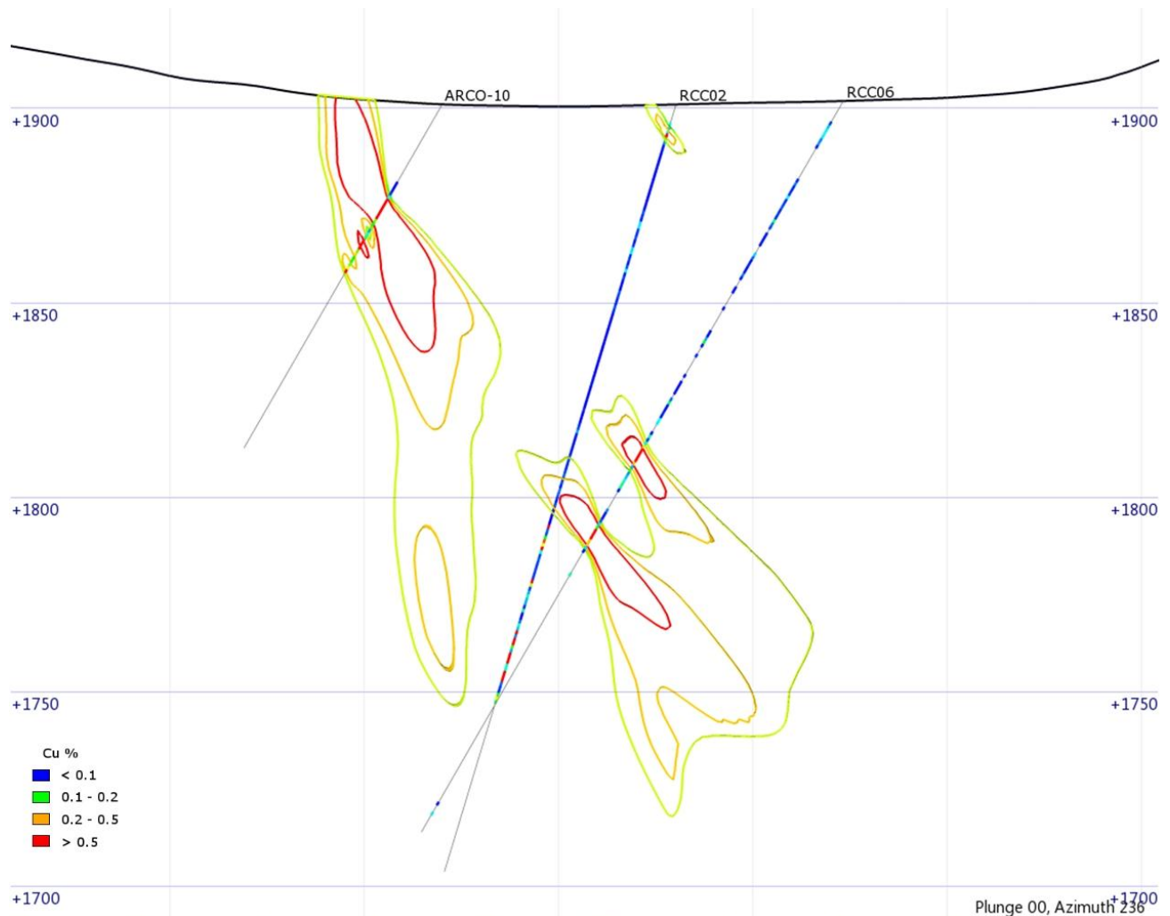
Figure 1: Oblique SE (left) to NW (right) trending cross section of hole RCC06 at Colupo with drill holes, average grade intervals and >0.5% Cu (red) and >0.2% Cu (purple) copper mineralisation shells (see Figure 2 for cross section line location) (Datum PSAD1956 zone 19s).
