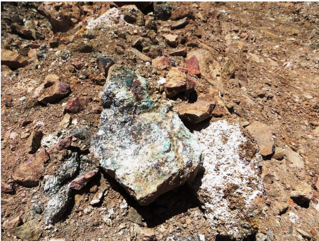
Figure 7 - Copper oxide mineralisation with limonitic, haematitic and sericitic alteration within trenches at Colupo Norte Prospect (January 2014).
