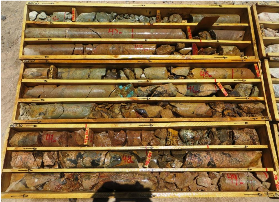
Figure 3 - HQ diameter diamond core from hole DHC-01 at Colupo identifying copper mineralised breccia intercept at approximately 43 metres to 51 metres downhole (January 2014).
