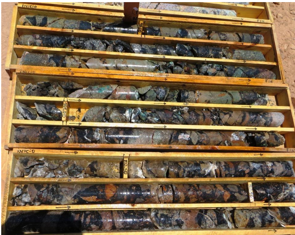
Figure 4 - HQ diameter diamond core from DHC-02 at Colupo identifying intercept 97 metres to 104 metres with visual extensive tourmaline filled breccia with copper mineralisation (January 2014).
