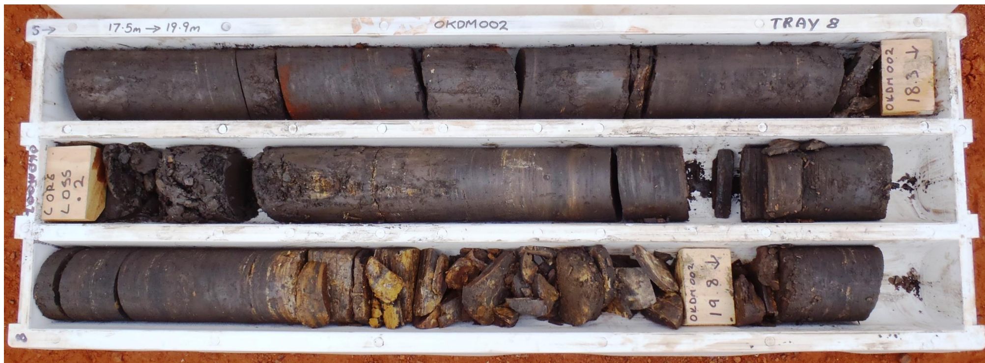
Photo 2: Diamond core hole OKDM002 17.5m to 19.9m. Massive manganese with minor manganiferous shale logged from 16.7m to 20.8m (see Photos 1 and 3).
