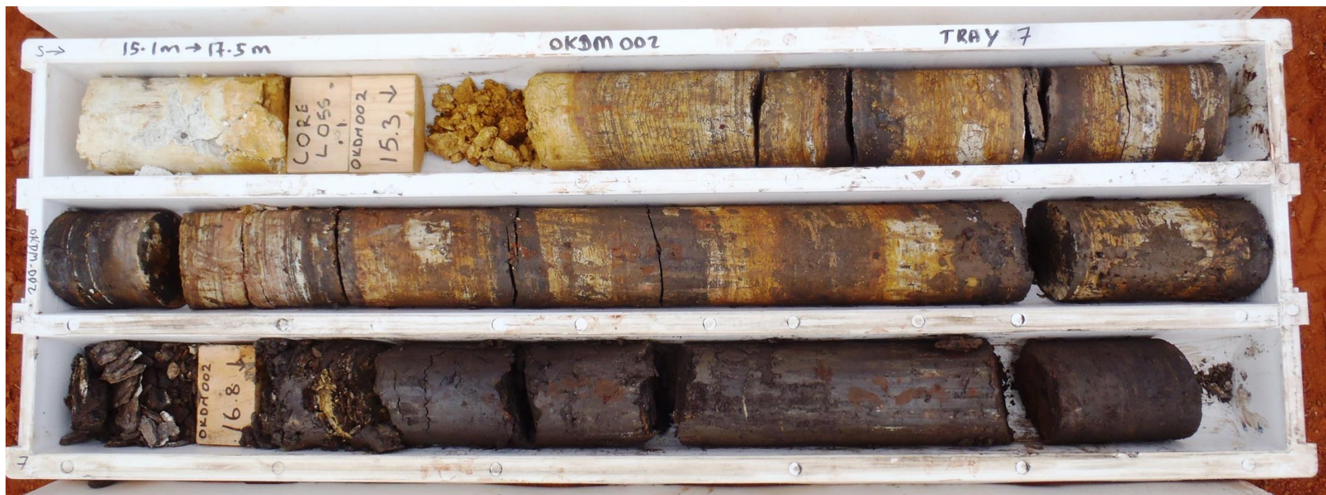
Photo 1: Diamond core hole OKDM002 15.1m to 17.5m. Massive manganese with minor manganiferous shale logged from 16.7m to 20.8m (see Photos 2 and 3).
