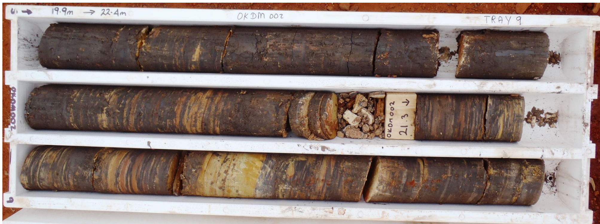
Photo 3: Diamond core hole OKDM002 tray 19.9m to 22.4m. Massive manganese with minor manganiferous shale logged from 16.7m to 20.8m (see Photos 2 and 3).
