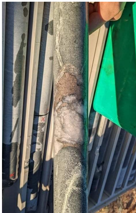
Figure 1: Photo showing remobilised sulphides (dominantly nickeliferous pyrrhotite and quartz with minor chalcopyrite) from TXDD002 from ~142m (L) and from ~137m (R).
