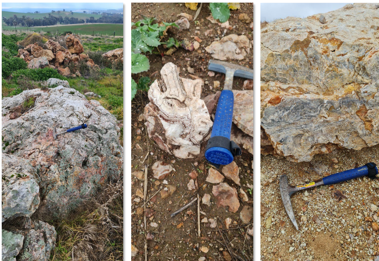
Figure 1: Vein outcrop and float from across the Bauloora Project showing sinter related veins and crustiform-colliform banded textures typical of low-sulphidation epithermal systems. The textures show dominant light and dark grey chalcedonic-quartz banding with yellow to light brown oxides after possible carbonate.
