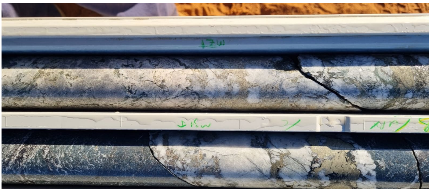
Figure 8-1: Drill core used for metallurgical studies
