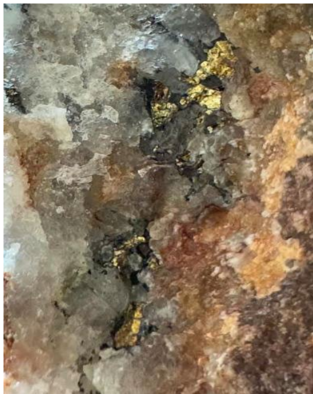
Figure 14 Chalcopyrite (ore zone) in quartz comb textures ('Bullseye Project porphyry').
