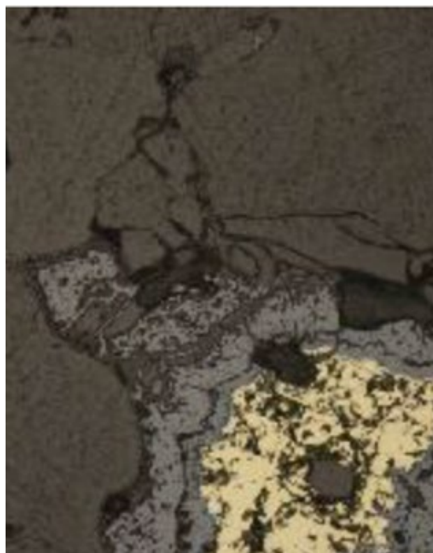
Figure 15 Petrographic analysis of Company sample showing copper mineralisation.
