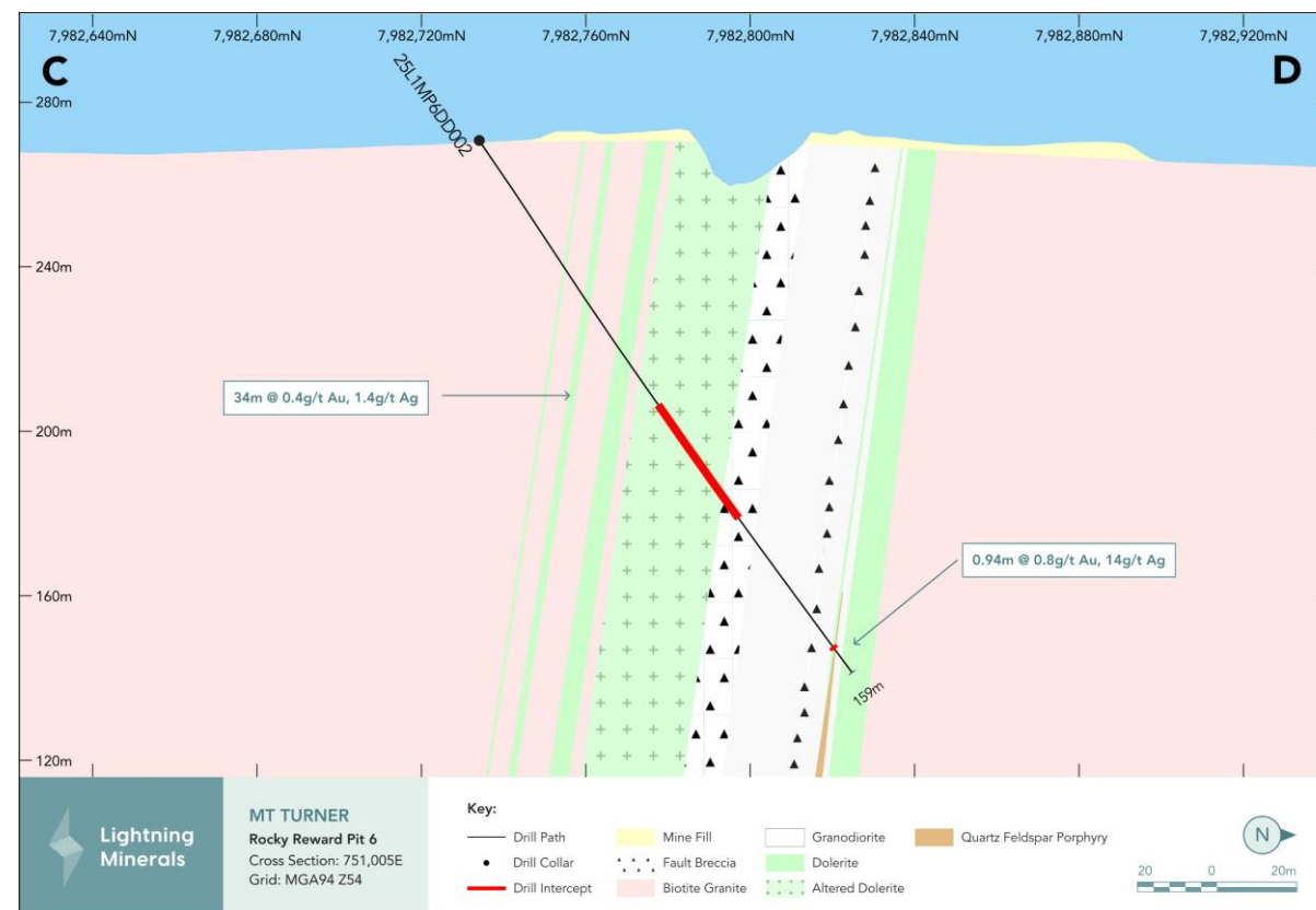
Cross-section of Hole 25L1MP6DD002 (Rocky Reward – Pit 6)
