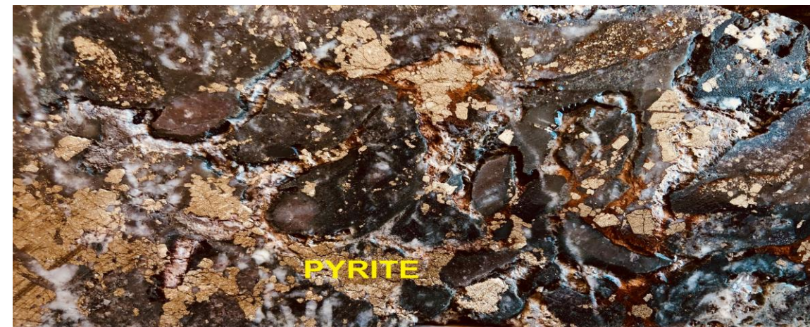
Epithermal breccia mineralisation (79.4m, Drill Hole 25L1MP3DD001) A
