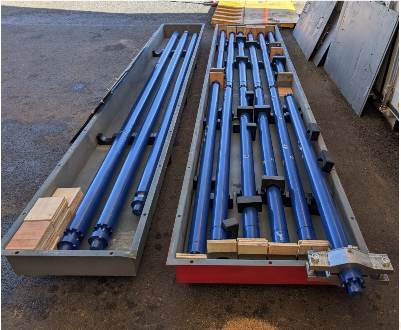
Electric Submersible Pump (ESP) for Ramsay 1 and Ramsay 2 well flow test rated to a maximum fluid flow rate of 2,000bbl/day undergoing factory acceptance tests
