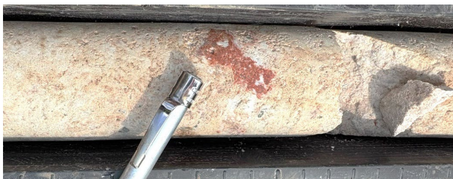
Figure 4 - Carbonatite drill core from approximately 449m downhole in 26NH032, showing textural variation and locally developed red-orange mineral/alteration phases. Mineral identification remains subject to detailed logging and analytical confirmation.
