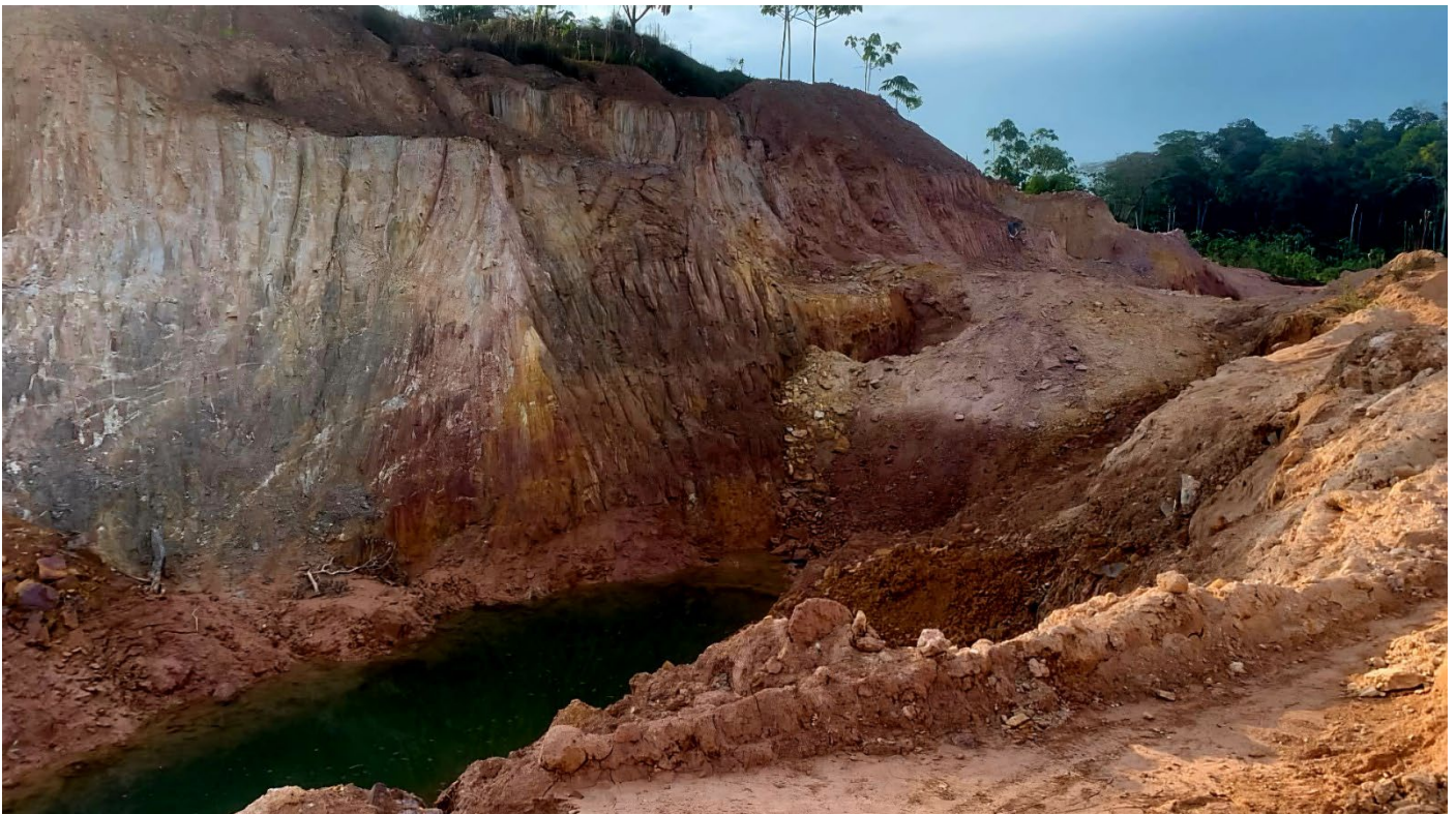
Figure 3 – Third-party small-scale open pit on the Gadu Manda right, exposing the deep tropical weathering profile (photograph circa 2026). The workings are operated by third parties, not by the Vendor or the Company.
