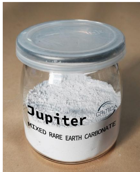
Figure 22: Representative MREC sample produced from Jupiter mineralisation by GAVAQ. Final analytical results are pending.
