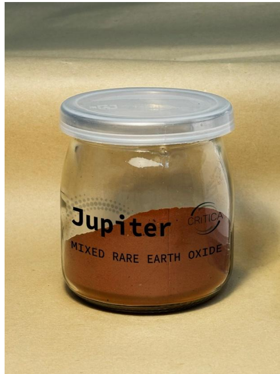
Figure 21: Representative MREO produced from Jupiter mineralisation as part of the Company's metallurgical and product-development programmes. The MREO grades 98.2% TREO, of which 28.4% comprises the four principal magnet rare earth oxides (Nd, Pr, Dy and Tb).
