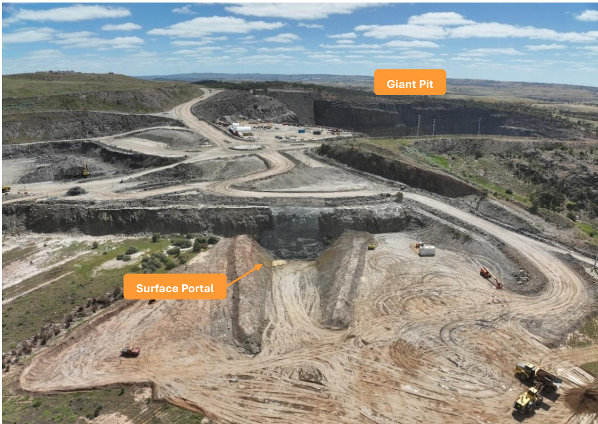
Figure 3: Surface Portal to Emily Star under development
