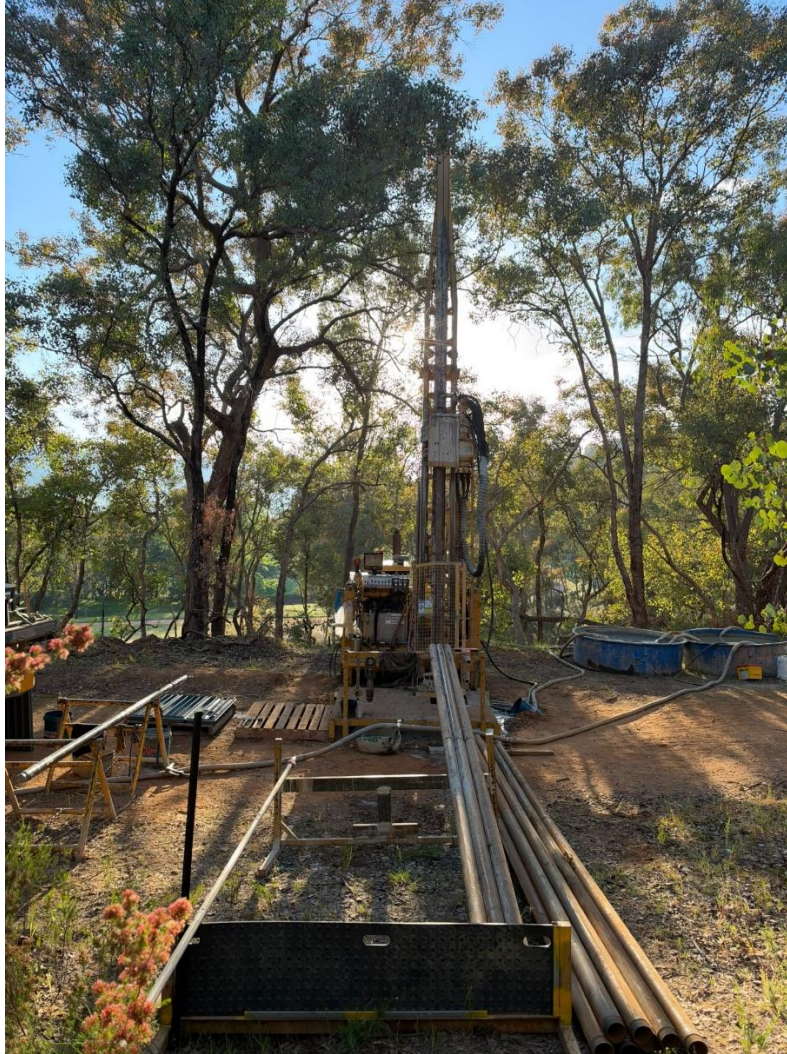
Figure 2 – Diamond drilling has commenced at Walwa – first core in trays to left of rig
