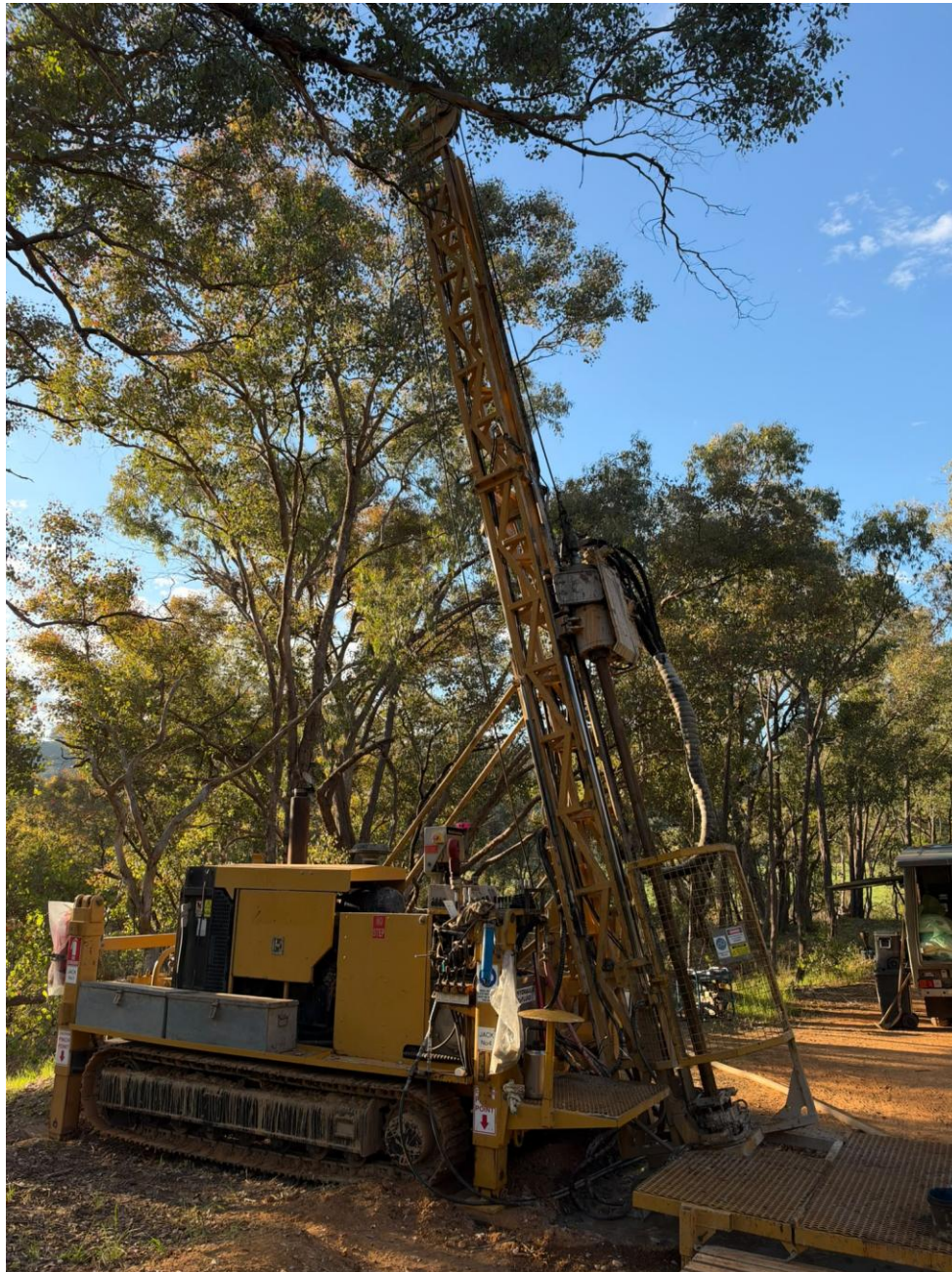
Figure 1 – Dart’s diamond drilling set up ready to commence drilling at Walwa
