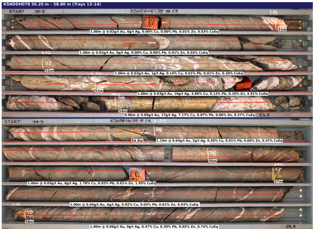
Figure 6: Massive sulphide intersection in KSNDH078 drill core. The intersection from 54m contains massive chalcopyrite mineralisation and abundant quartz veining. This intersection aligns with the surrounding intersections of the main D Lode structure.
