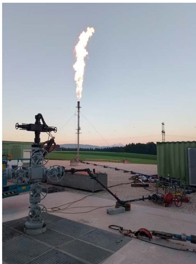
Testing at the HOCH-1 shallow gas discovery well in Upper Austria
