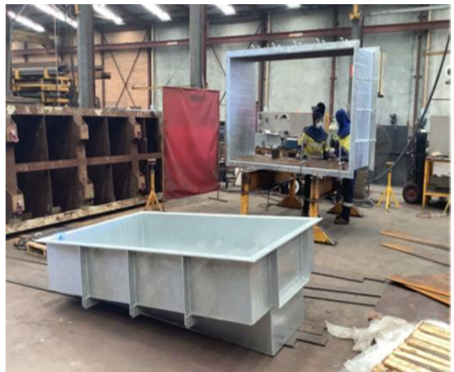
Figure 2: Workshop Fabrication of Steel Tank Components
