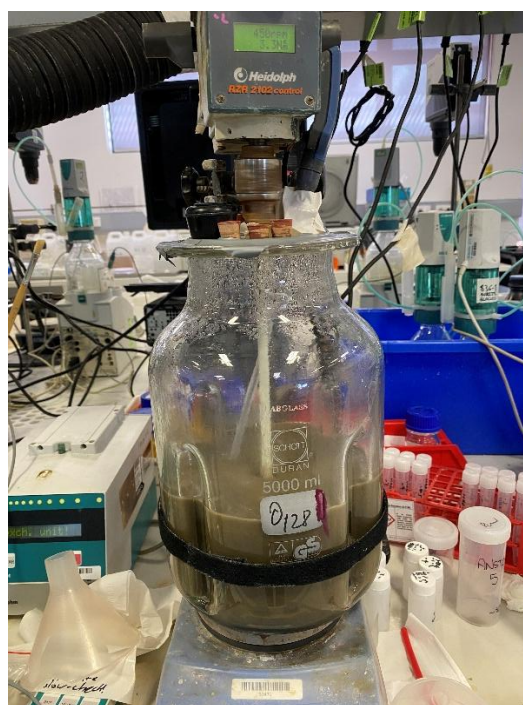
Figure 6: Profile leach testwork is underway at ANSTO.
