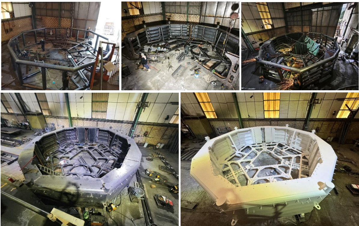
Fabrication snapshots of the ACHIEVE CETO Buoyant Actuator over recent months
