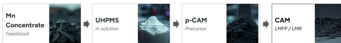
Figure 7: Firebird's proprietary and integrated lithium manganese rich (LMFP & LMR) cathode process commences with the production of ultra-high-purity manganese sulphate (UHPMS).
