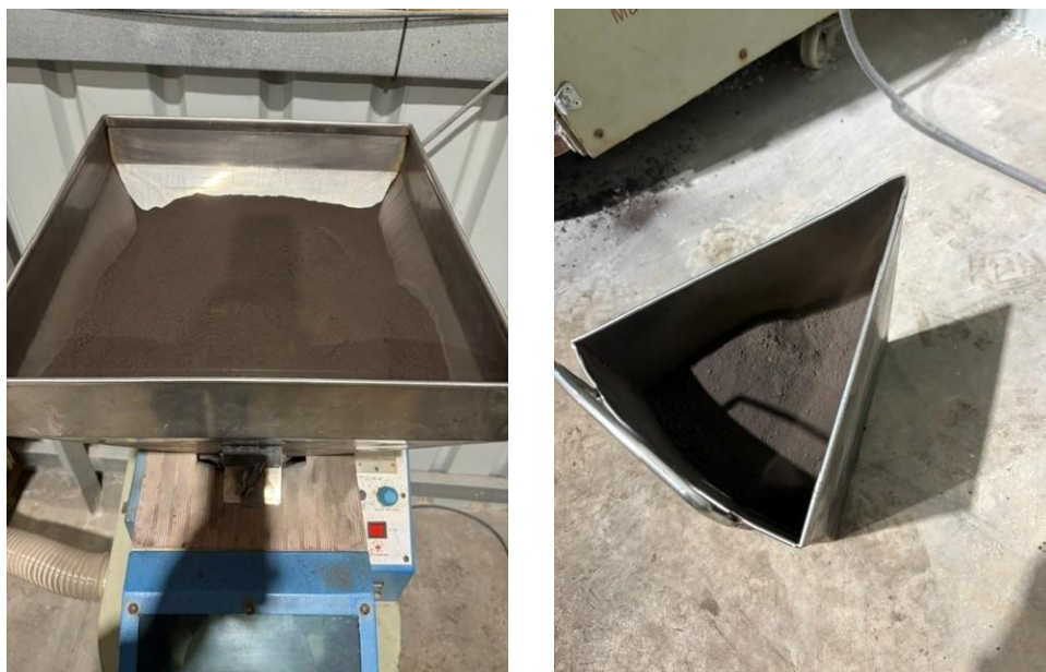
Figure 5: Milled Oakover manganese ore prepared as first feedstock for the ADP.
