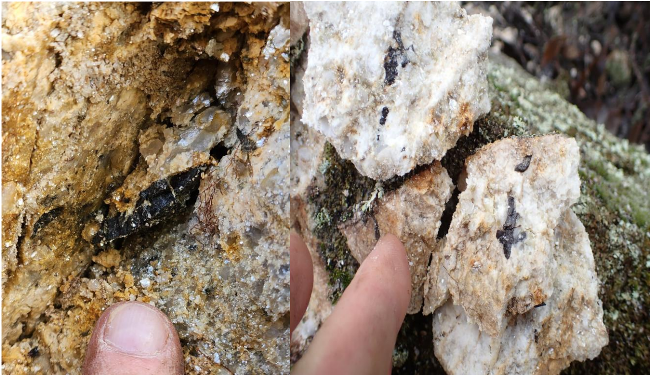
Figure 5: Walwa rock chip samples - Top left: Sample WWP002 (3.96% Sn) - coarse black cassiterite in pegmatite from the south-west wall of the historic Walwa open pit. Top right: Sample WWP001 (1.09% Sn) - cassiterite in a greisenous pegmatite boulder from the floor of the historic Walwa open pit. Bottom left: Sample WWP003 (0.61% Sn) - cassiterite in coarse aplite-pegmatite from outside the northern pit wall. Bottom right: Sample WAS001 (0.40% Sn) - from the Mt Alwa South dyke.
