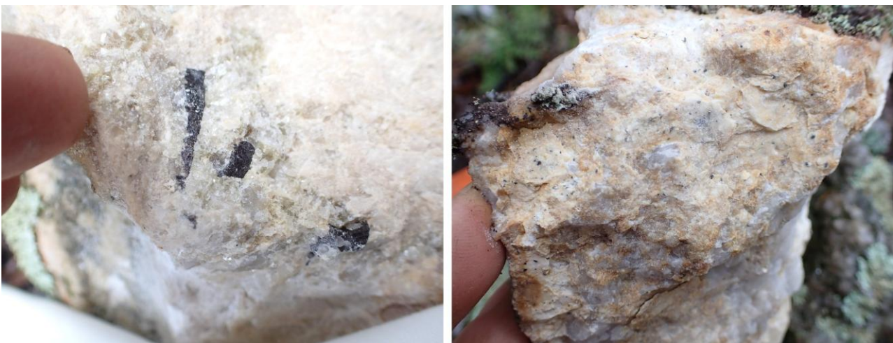
Figure 5: Walwa rock chip samples - Top left: Sample WWP002 (3.96% Sn) - coarse black cassiterite in pegmatite from the south-west wall of the historic Walwa open pit. Top right: Sample WWP001 (1.09% Sn) - cassiterite in a greisenous pegmatite boulder from the floor of the historic Walwa open pit. Bottom left: Sample WWP003 (0.61% Sn) - cassiterite in coarse aplite-pegmatite from outside the northern pit wall. Bottom right: Sample WAS001 (0.40% Sn) - from the Mt Alwa South dyke.
