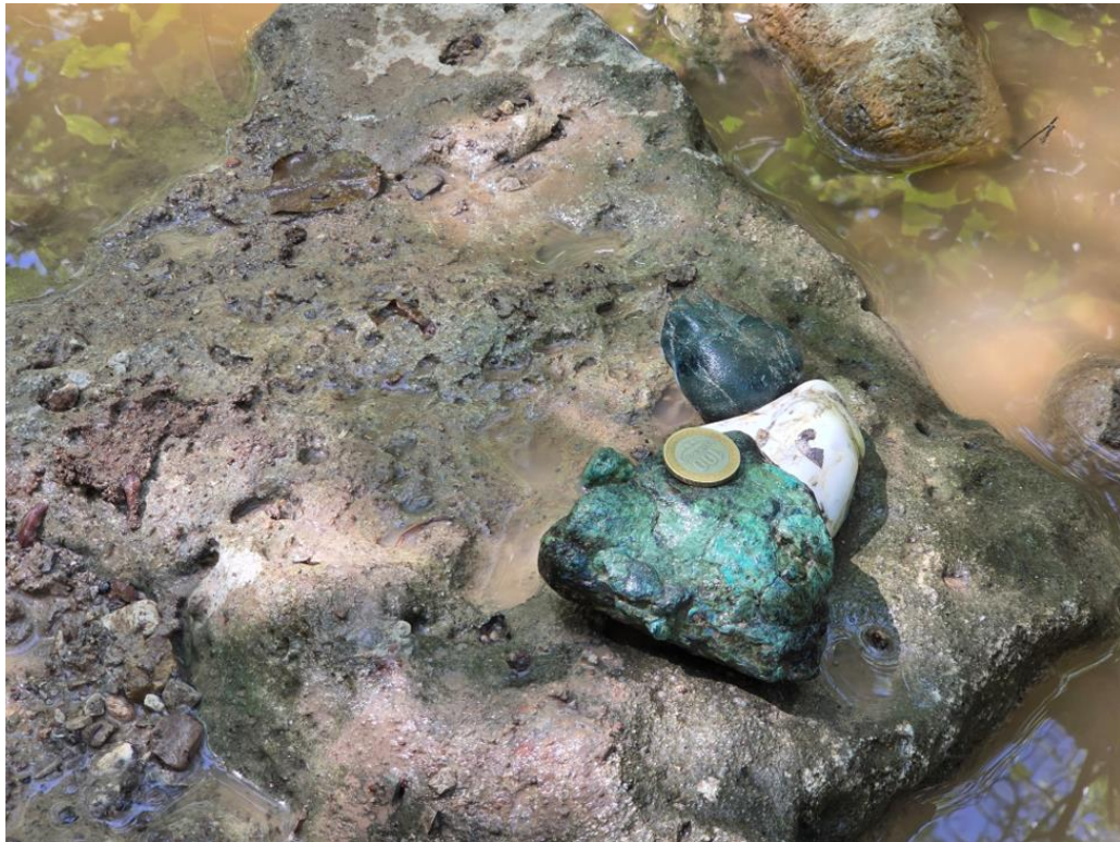
Figure 3: Specimen of oxidised copper-bearing massive sulphide, sampled as ESR006095, which assayed 60.34% Cu
