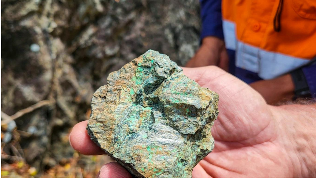
4 Figure 6: Example of copper mineralisation* within hydrothermally altered porphyritic rock, sampled as ESR006498. The copper mineralisation consists of malachite films on fracture surfaces and occurs as a trace through to 1-2% of the rock mass.
