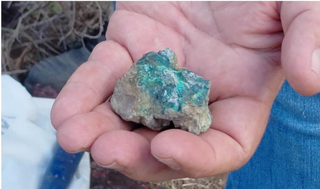
Figure 9: Portion of sample ESR006489, comprised of malachite * (~ 5%) as films on a matrix of magnetite (10-15%), goethite (60-70%) and quartz (20-30%). 4
