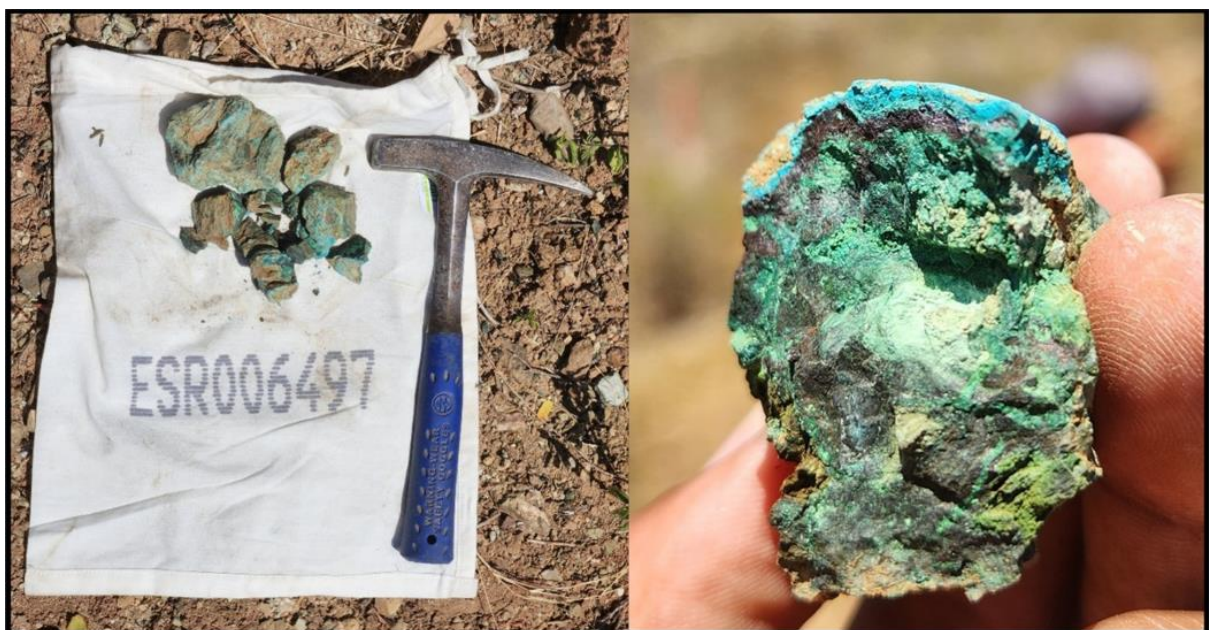
Figure 7: Sample ESR006497; left image shows exterior appearance, dominated by pale blue chrysocolla*, while the right image shows the chrysocolla is surface skin overlying an interior of bright green malachite, brown goethite, along with an unknown yellow-green mineral and grey silica. 4
