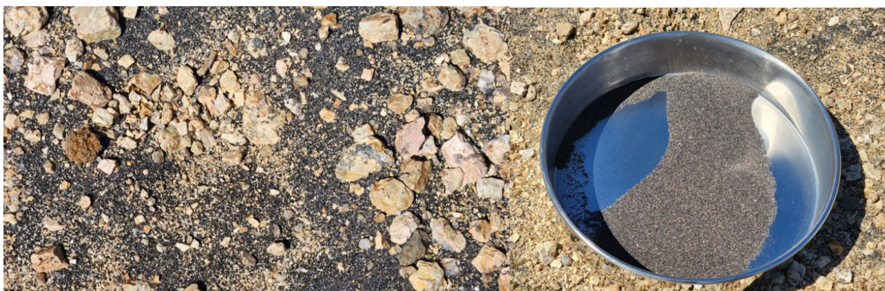
Figure 5. Concentrations of naturally occurring heavy mineral sands identified within eastern drainage systems and beach foreshores and sieved heavy mineral concentrate (<200 \mu\text{m} ) collected from eastern drainage systems for laboratory analysis.
