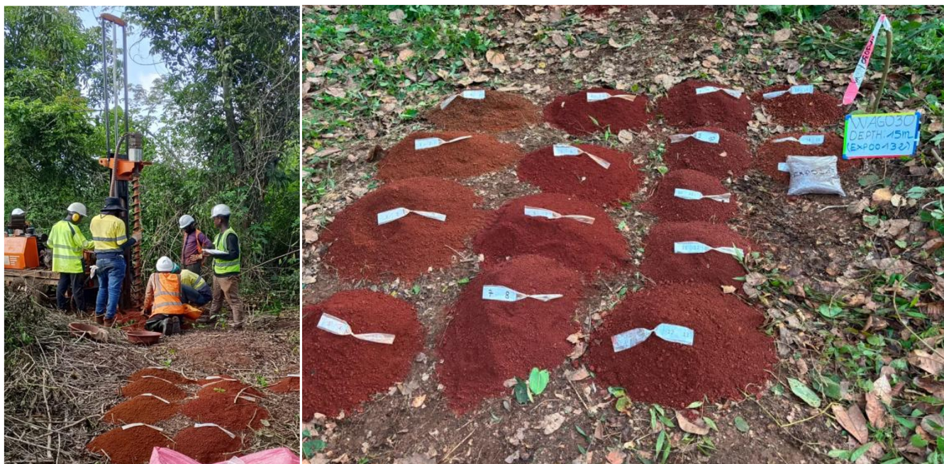
Figure 1. Auger drilling being conducted.
