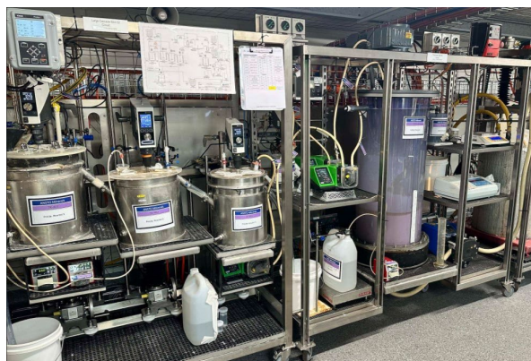
Continuous three-stage precipitation reactor with MREOH accumulating in transparent thickener vessel (right).
