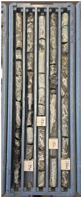
OV176 core (185m to 190m) showing pervasive carbonate veining, typical of carbonatites.
