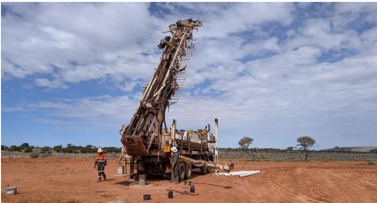
Figure 1: Hydrogeological drilling ongoing at Windabout.
