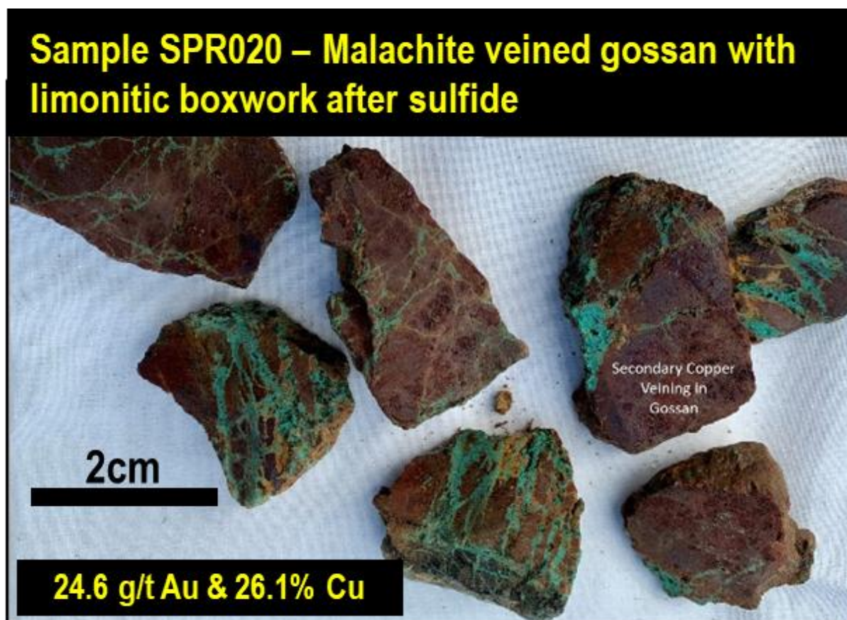
Figure 6: Mullock sample of malachite veined gossan with limonitic boxwork after sulfide (Sample SPR020) (ASX: SLZ 20 May 2020).
