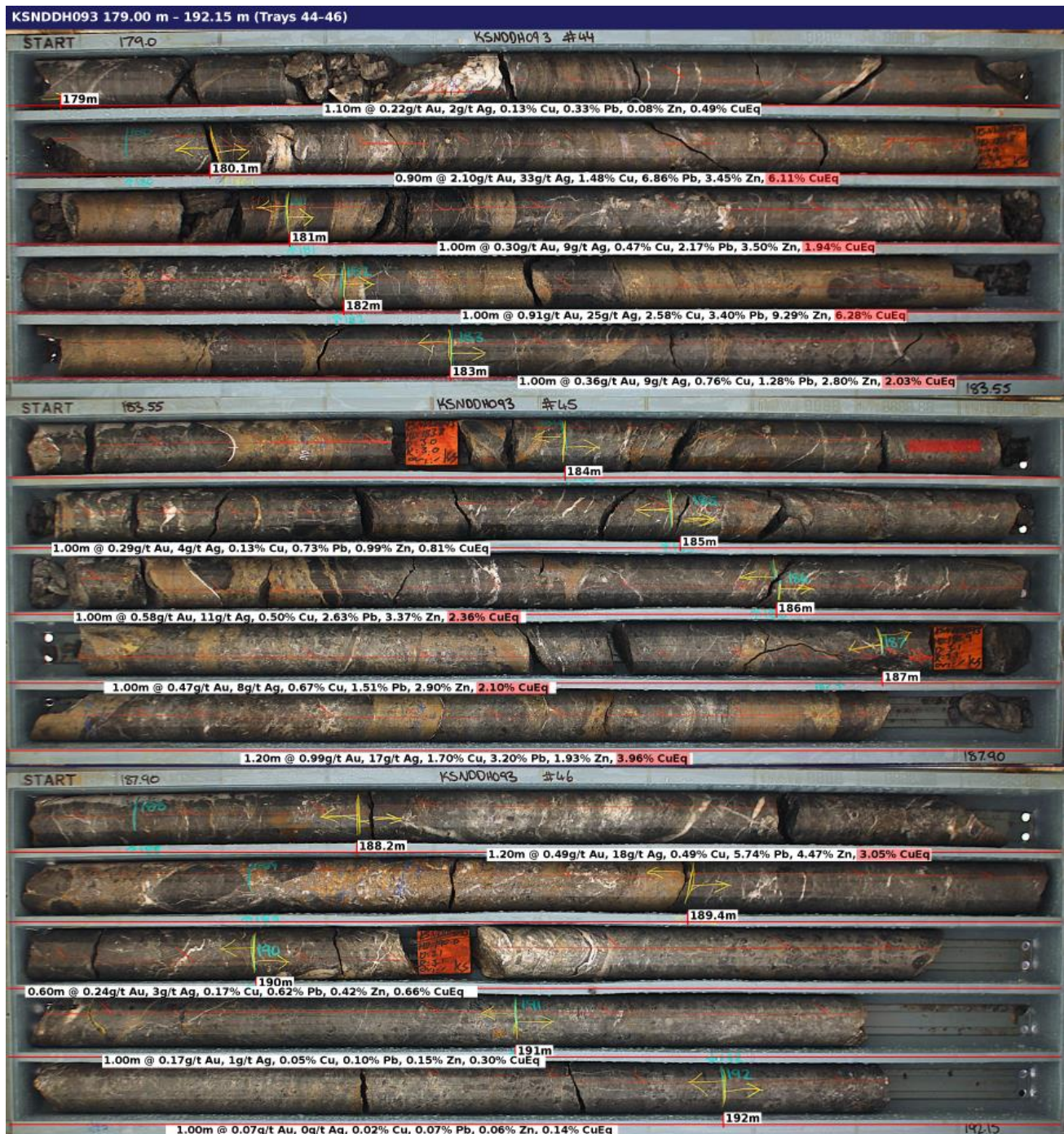
Figure 7: Core photos KSNDH093, 179m - 192.15m, showing chalcopyrite, galena, sphalerite mineralisation.
