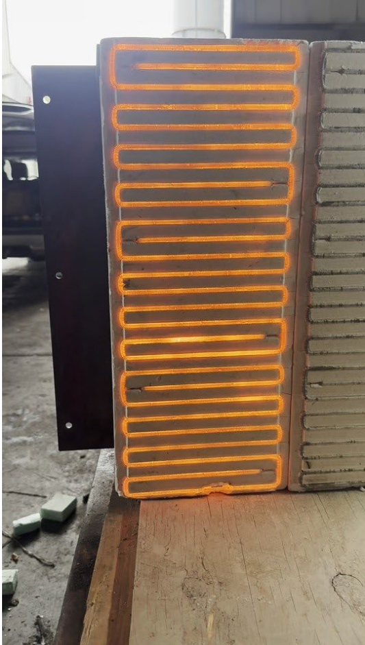
Heater element under test at operating temperature
