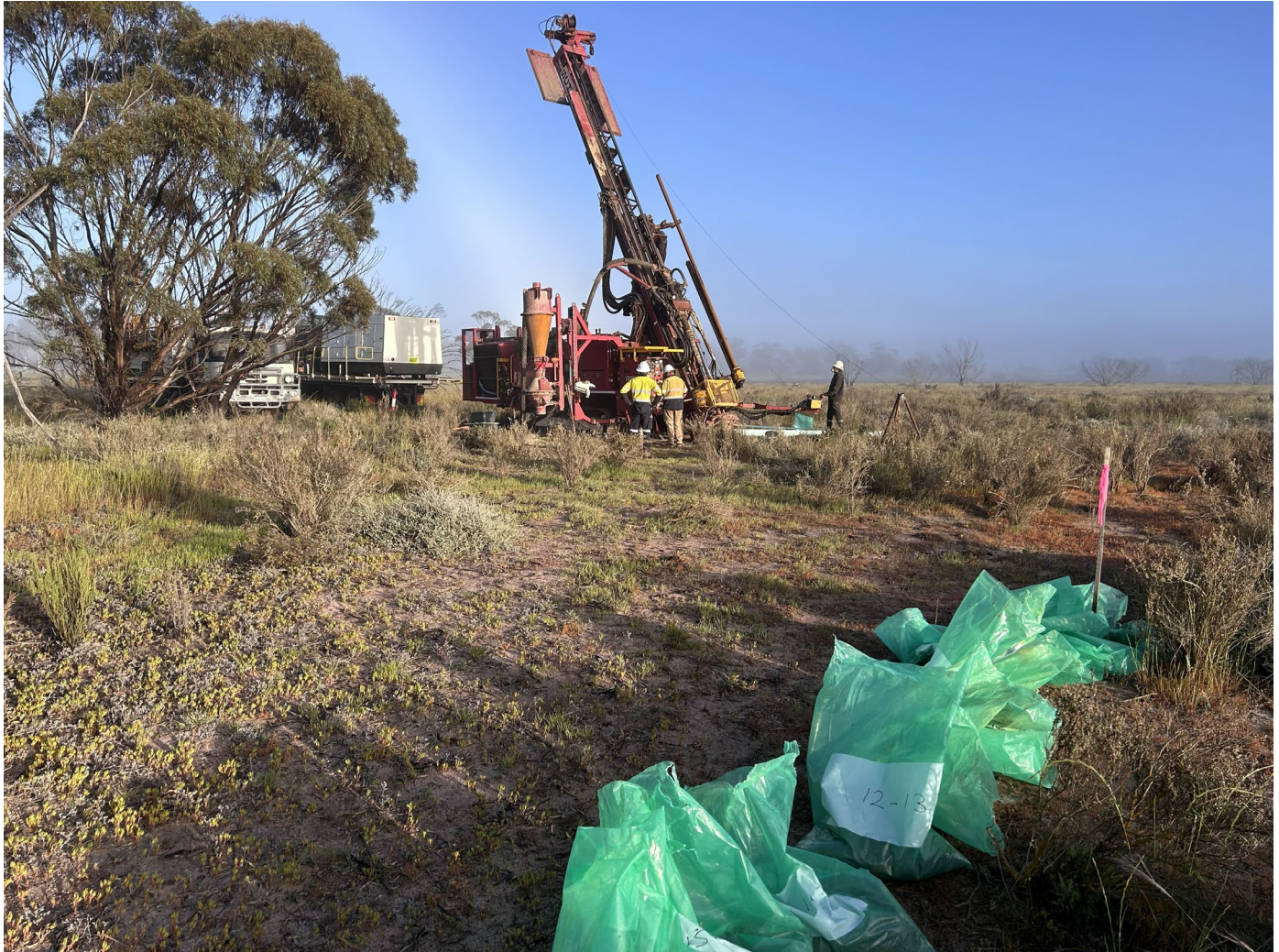
Figure 1: RC drilling at Bindi SW.
