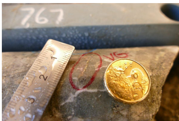
Image 3 (left): 26FRD001 core at ~767ft (233.8m) downhole showing a visible native gold veinlet extending for more than 1cm, logged after quarter end; this interval returned 0.39m @ 120.0 g/t Au 1 . Scale shown in cm/mm with a 20.5mm diameter coin. Image 4 (right): CEO Edward Keys and geologists inspecting 26FRD001 core at Friday.
