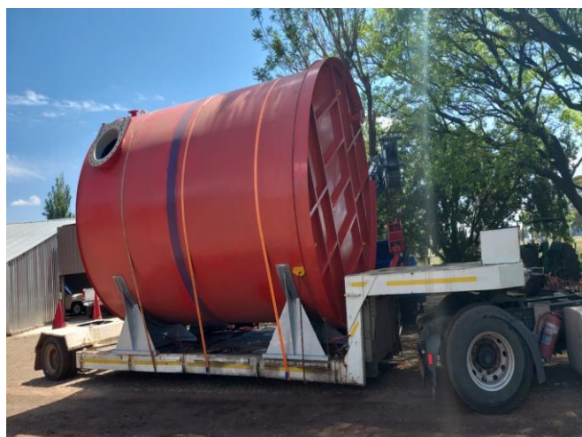
Figure 10: Cyanide Tank fabrication and delivery to site
