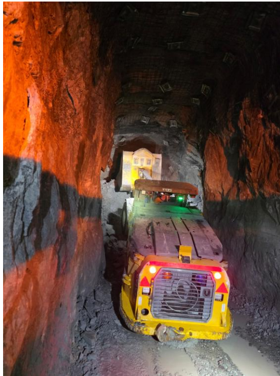
Image 12: Stopes are bogged using the remote-controlled Aramine loaders
