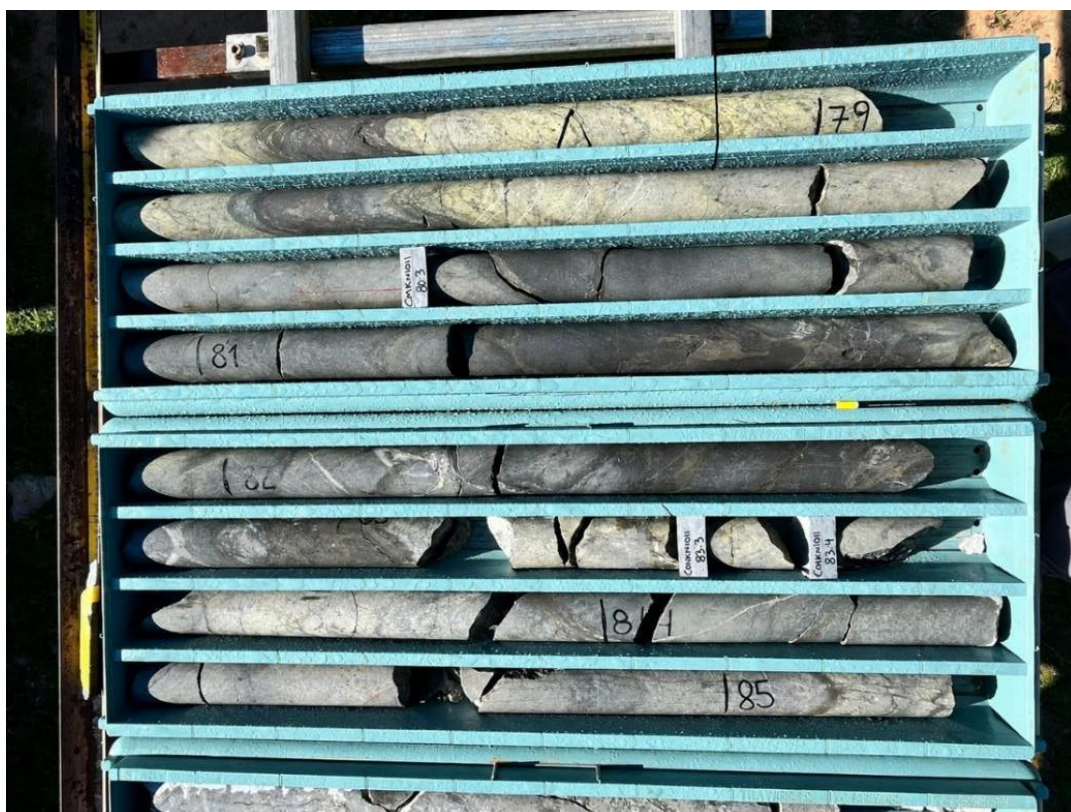
Figure 4. Diamond drill core from CMKNI011 showing 20–50 cm thick sulphide veins in silica-sericite altered rhyolite at Silica Hill.
