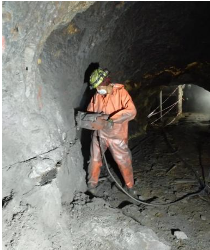
Figure 6: Collection of bulk sample from lower graphite layer as exposed in the former graphite mine using a diamond blade saw to cut sampling channels.
