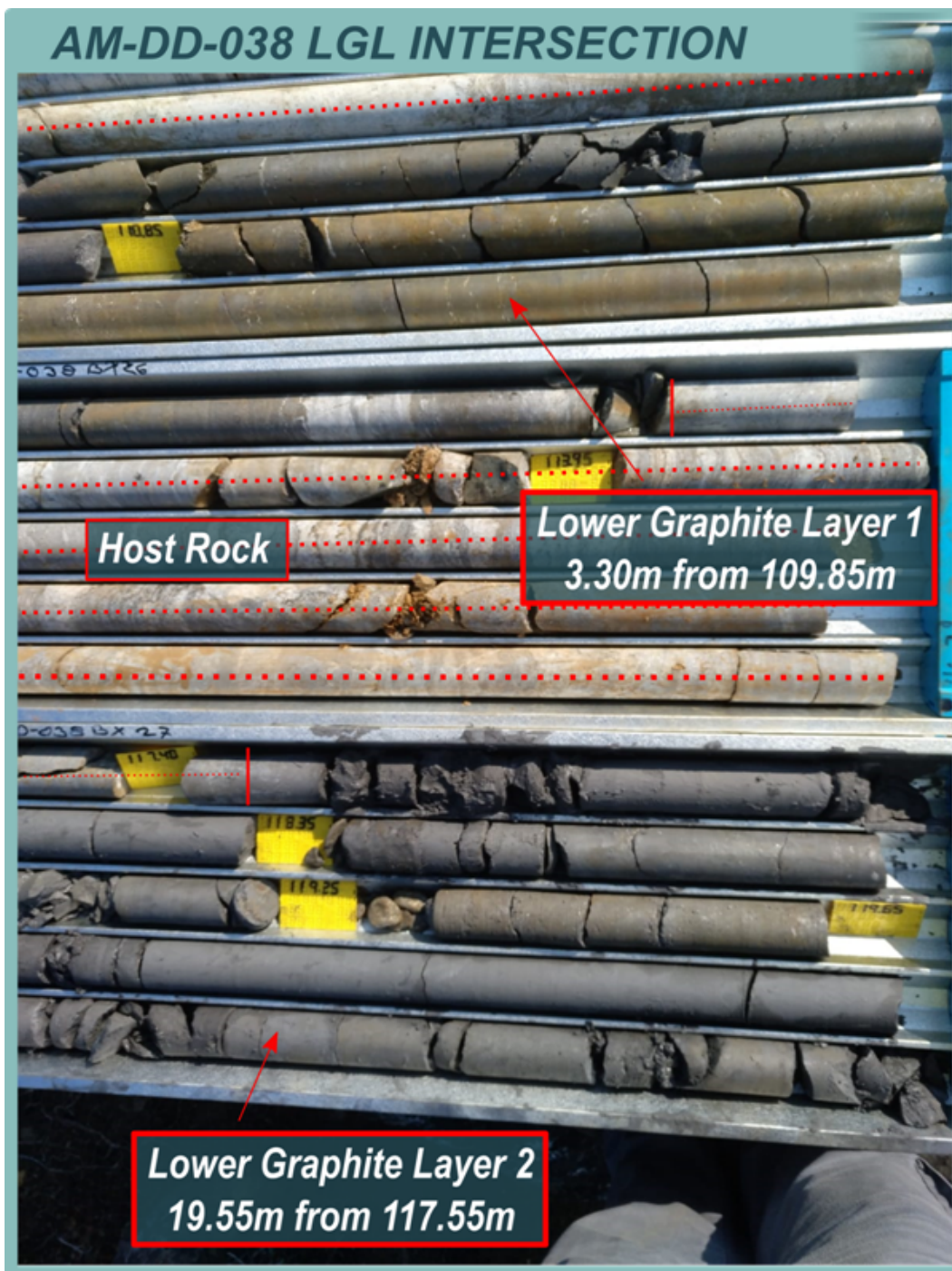
Figure 5: Drill core from AM_DD_038 showing part of the intersections of LGL1 of 3.30m (3.10m true thickness) and LGL2 of 19.55m (18.36m true thickness). Note the abrupt shift in colours from the light grey gneiss forming the wall rocks to the black graphite-rich ore.
