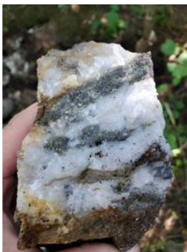
Photo 1 quartz vein from Sample 697925, assaying 7.02ppm Au, with minor pyrite and galena in sheared, silicified granodiorite containing 1-2% disseminated pyrite.
