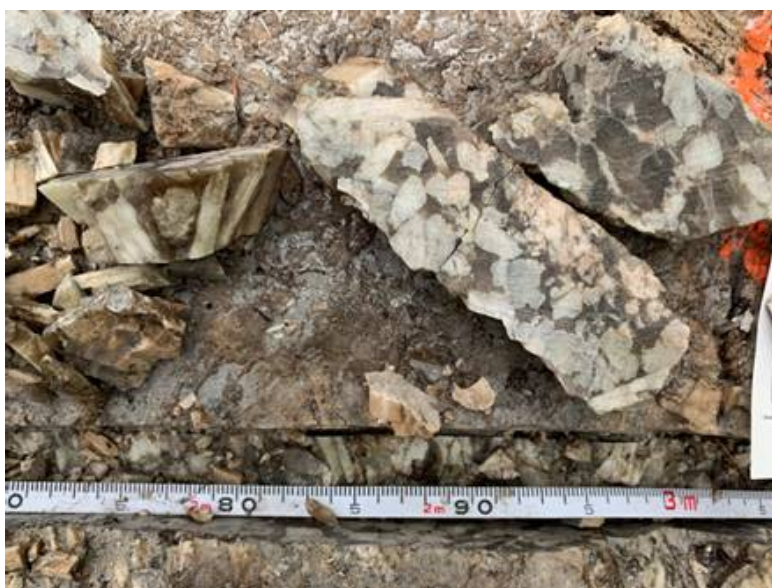
Photo 5 close up of sample from sawn channel. Note coarse spodumene crystals.
