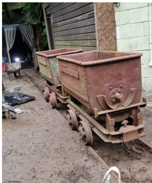
Above: Historic rail tracks and ore tubs rehabilitated for transport of blasted ore
