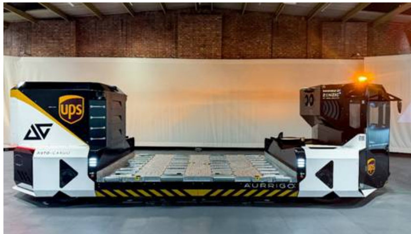
Image: Auto-Cargo®, an autonomous electric vehicle designed to move heavy cargo loads to and from aircraft
