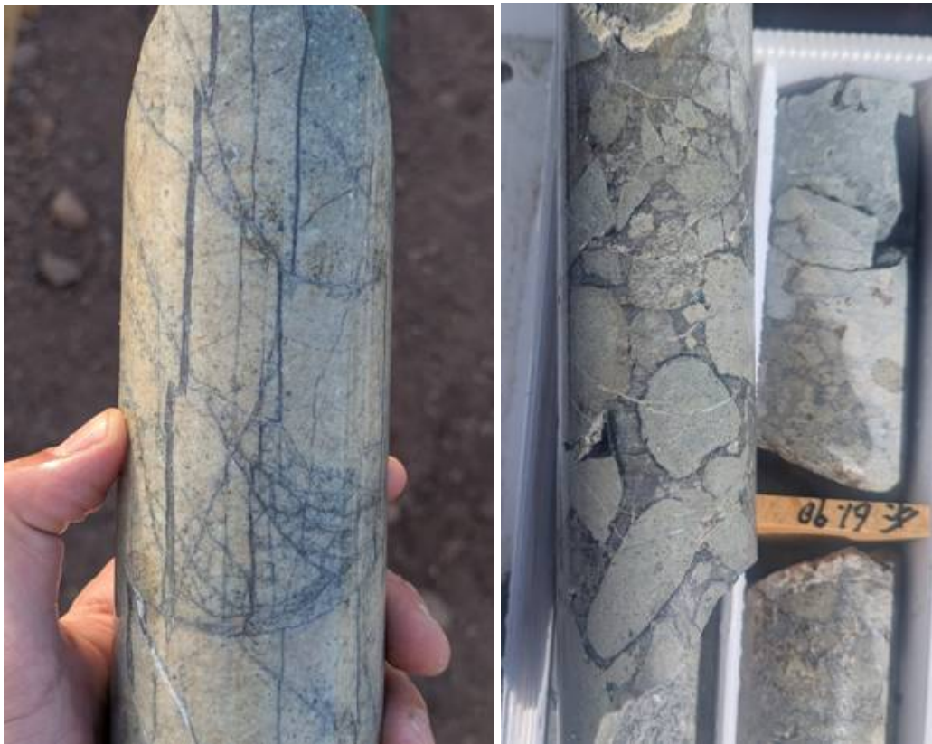
Figure 3: Drill core from VNE25-DD001 demonstrating Maricunga-style quartz fracture-veining (l) and hydrothermal brecciation (r).
