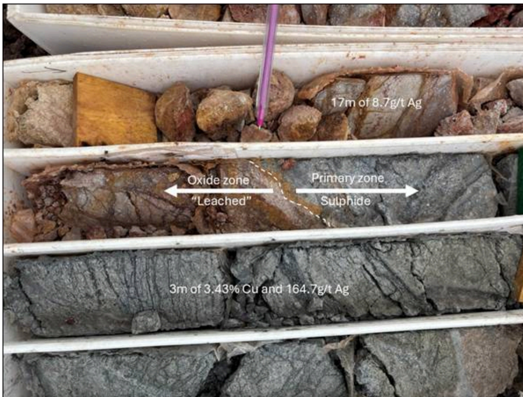
Figure 5: Hole CNG25 DD012, core illustrating the sharp transition from oxidised leached core (with anomalous silver) to primary, sulphide-rich lens material with high-grade copper-silver mineralisation at 24m depth down-hole.
