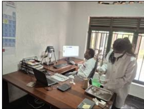
The Company's pXRF station for verifying delivered concentrate grade.
