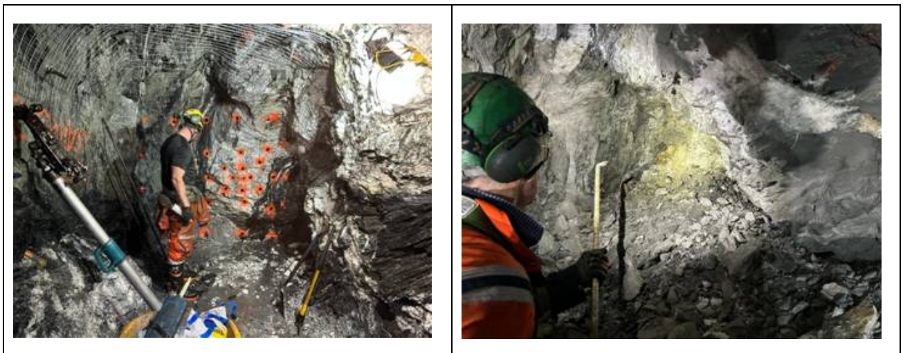
Figure 1: (Left) Completed blast holes for Blast 7; (Right) Ore pile post Blast 7.
