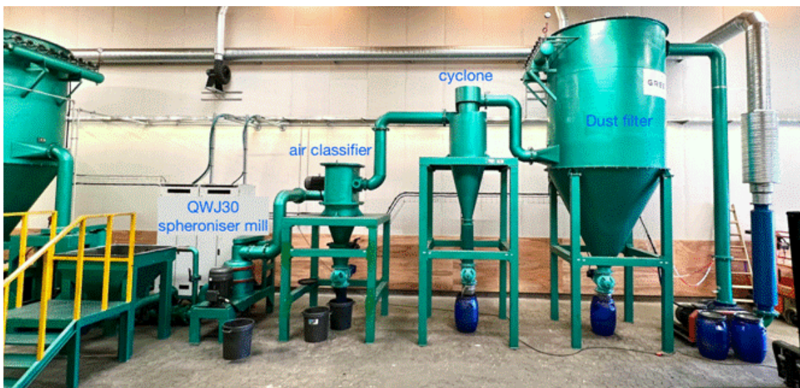
Figure 2. The spheronising mill line, with various air classifiers to separate spheronised graphite from fine-grained graphite by-products.
