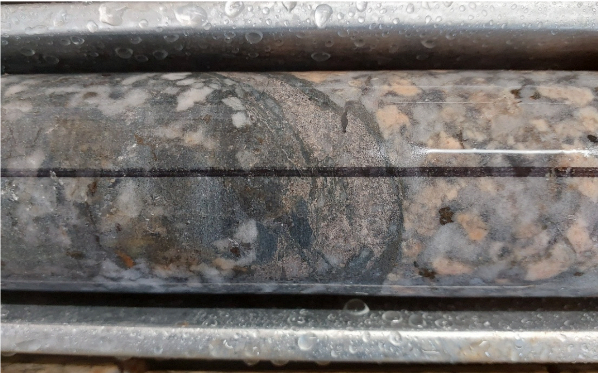
Figure 2: Quartz tourmaline vein hosted in granite with a band of cassiterite mineralization (e.g. indicated by the orange arrows), as logged by Cornish Metals geologists.
