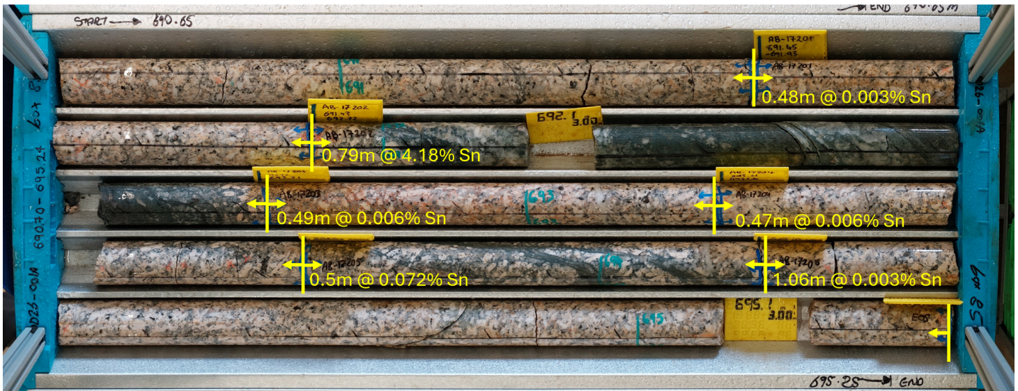
Image 2: Core tray image showing section interpreted to be Roskear 1 South lode; strong tourmaline-quartz-chlorite with disseminated cassiterite and well-defined hangingwall and footwall contacts
