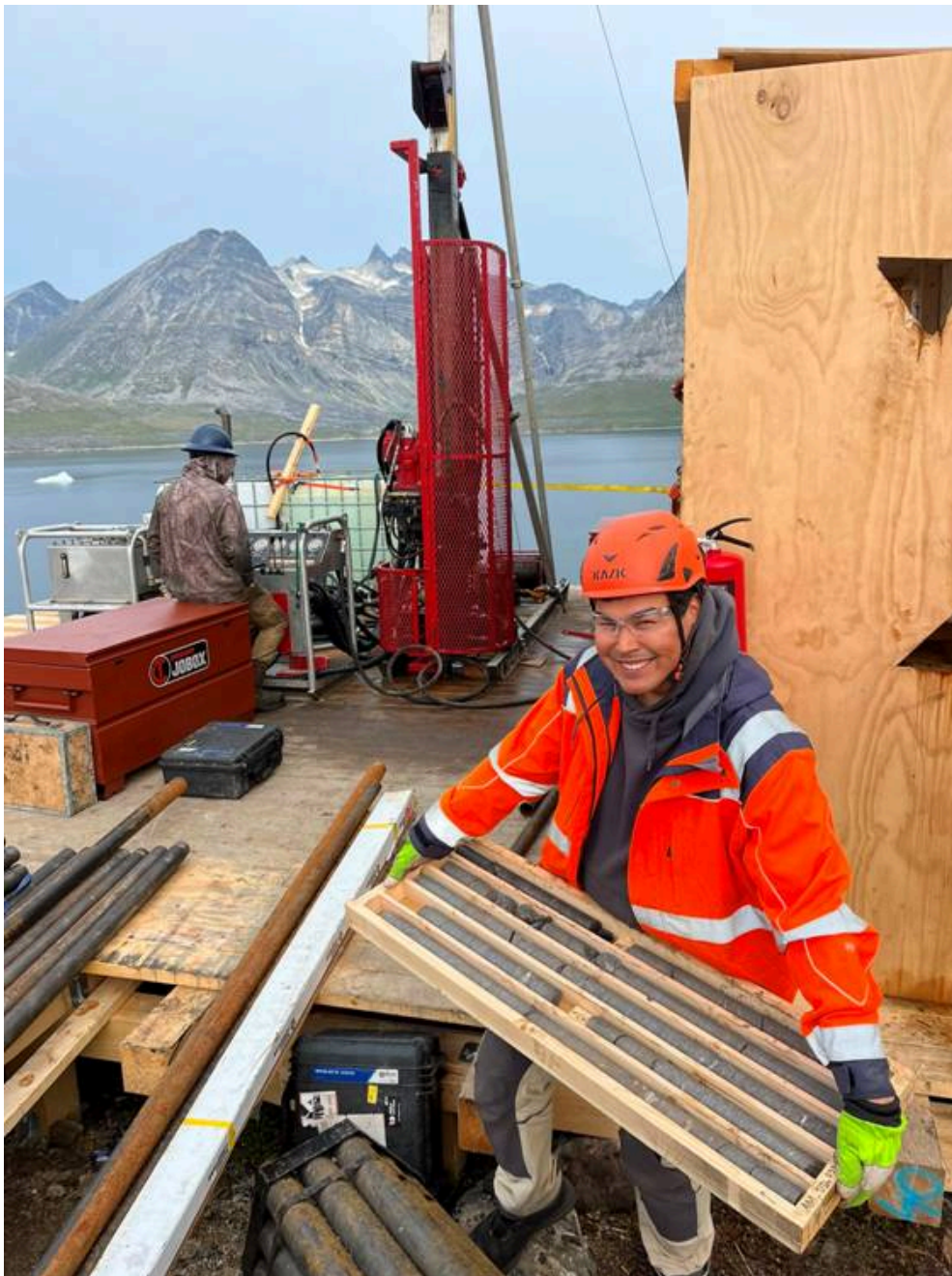
Figure 1. Drilling at Amitsoq conducted by drilling team from MEDL and a box of about 5m of drill core with Lower Graphite Layer ore intersection
