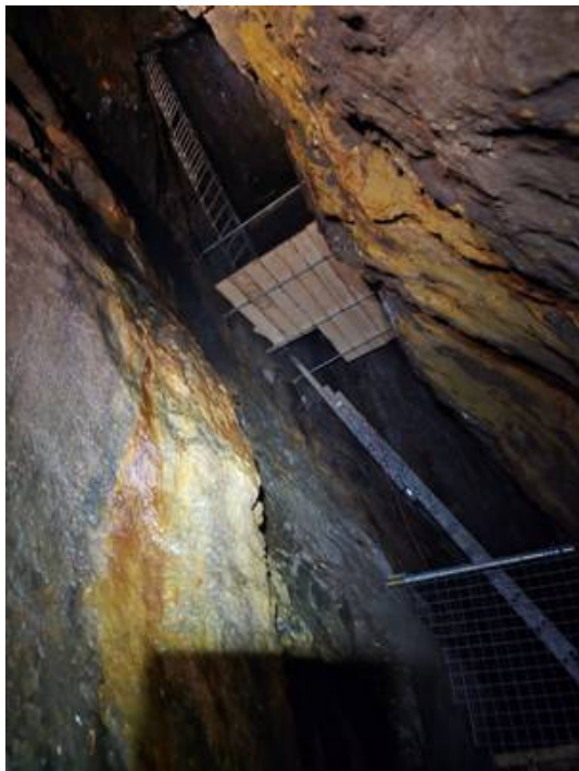
Figure 1: A section of the new ladders and platforms installed at the Jack Williams stope, Tyn y Cornel level.
