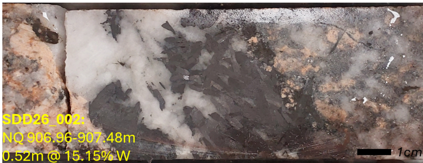
Photo 5: SDD26_002 Cut Core (907.0 – 907.5m) – Cross Section Reference G
