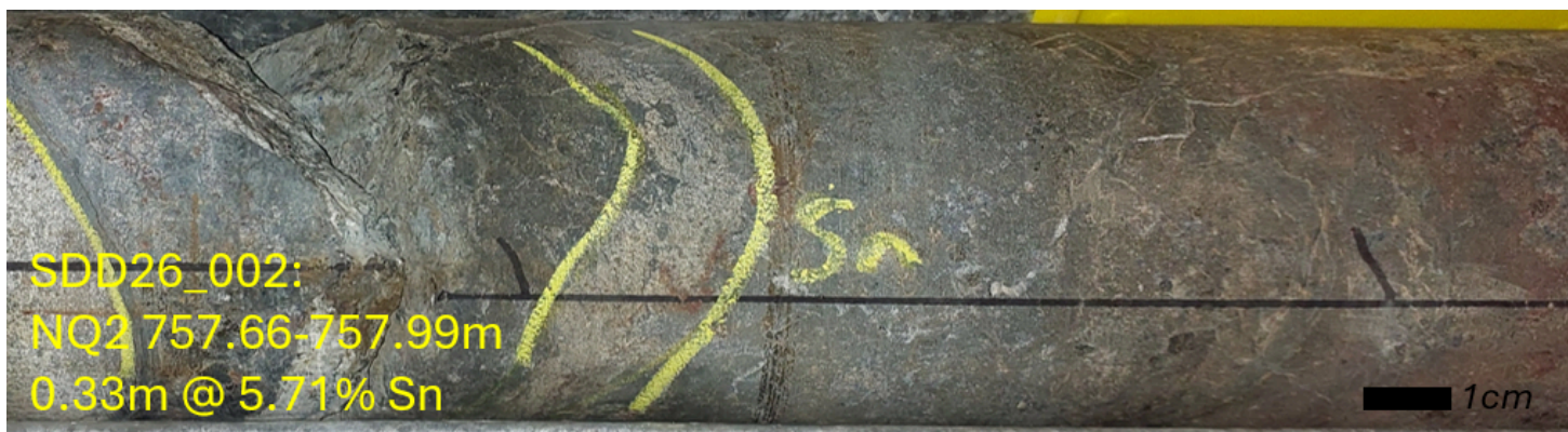
Photo 4: SDD26_002 Drill Core (757.7 – 758.0m) – Cross Section Reference C
